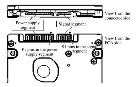
Figure 3.9 Power supply pins (CN1)
